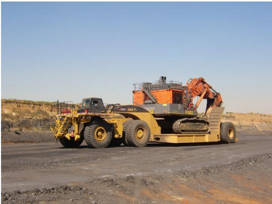
ETT Rear Loading Mining Lowbed Trailers provide efficient and safe mobility for tracked equipment – this 250T rigid model has the capacity to haul up to 250 metric tons.
