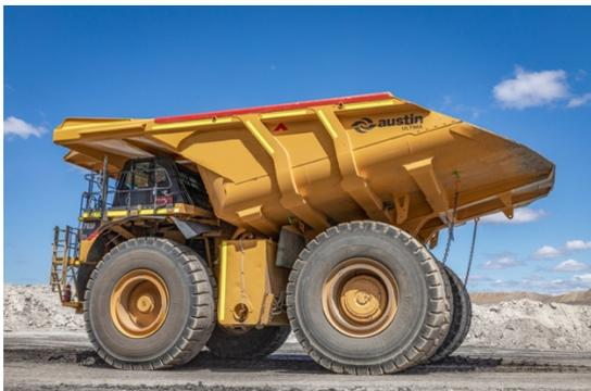
The Austin Ultima Dump Body – designed for more payload, providing longer life with special strength steels, and carrying Austin's 50+ years of innovation – offers the world's best lightweight dump body with more life, more payload for all OEM trucks.
