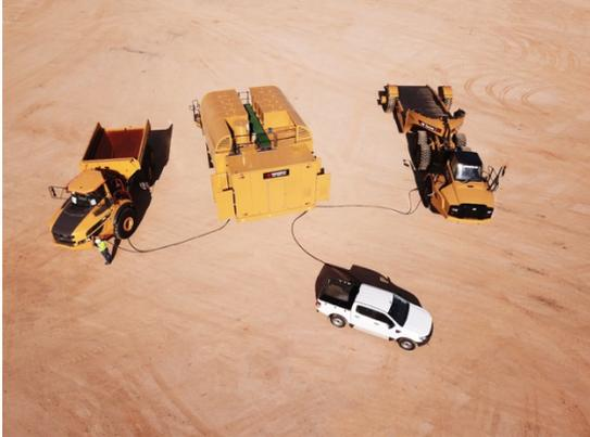
The dispensing systems of ETT's 100 Series Diesel Lube Truck are configured to customers' needs and are capable of filling three vehicles simultaneously.
